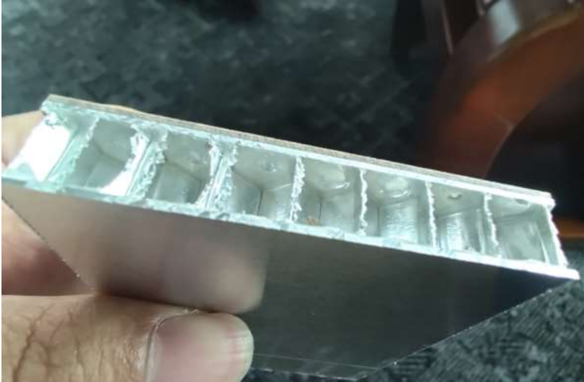
Laminated by hot melting film(PUR)
