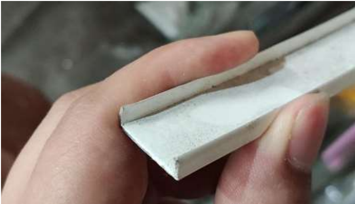
3.HPL strip (with insert reinforcement)
